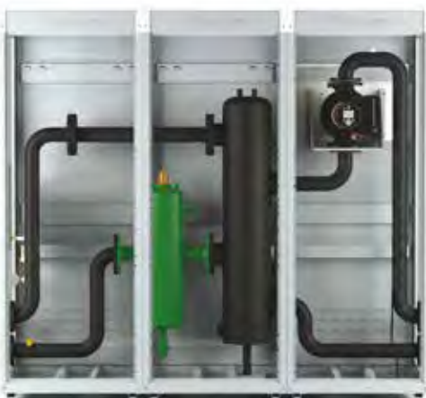
Grundfos Modulating pump max prevalence 15 m (with 15 m³/h of residual capacity) max capacity 55 m³/h (with 3 m of residual prevalence)
